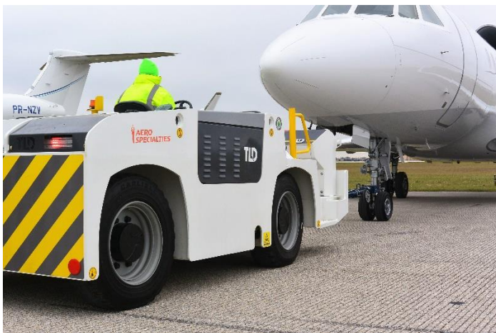
Taxibot: a pilot-controlled vehicle to taxi the aircraft with main engines off
